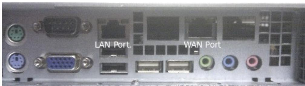
The SARK1200 has two (2) RJ45 Ethernet ports assigned as follows (when viewed, left to right, from the rear of the enclosure);
