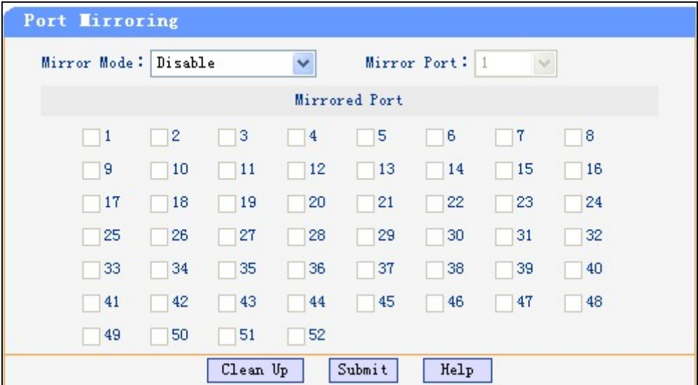
Figure 3-33 Port mirroring setting screen
