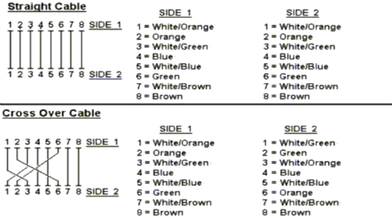
Figure A-1: Straight-Through and Crossover Cable
