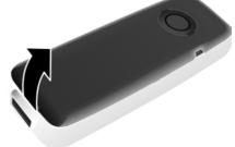
To **change the battery**, place your fingernail in the cavity on the casing and pull the battery upwards.
