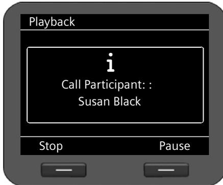
By default, call records are played back via the speaker. If a headset is connected, you can listen to the playback through this. If you pick up the receiver, you can listen to the playback through this.
